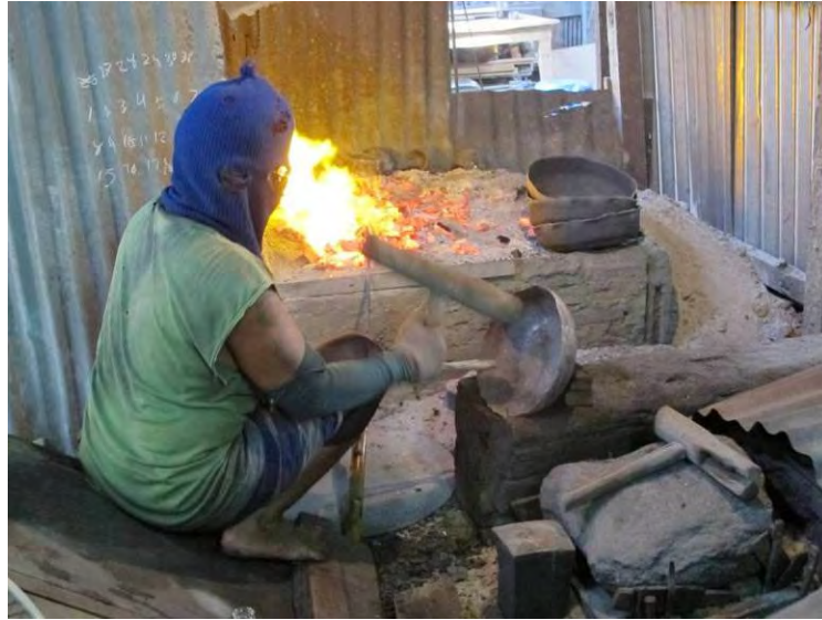
Figure 25: The forming craftsman is beating metal to form a shape of water jar
