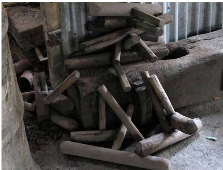
Figure 27: Wood hammers and the wood molds
