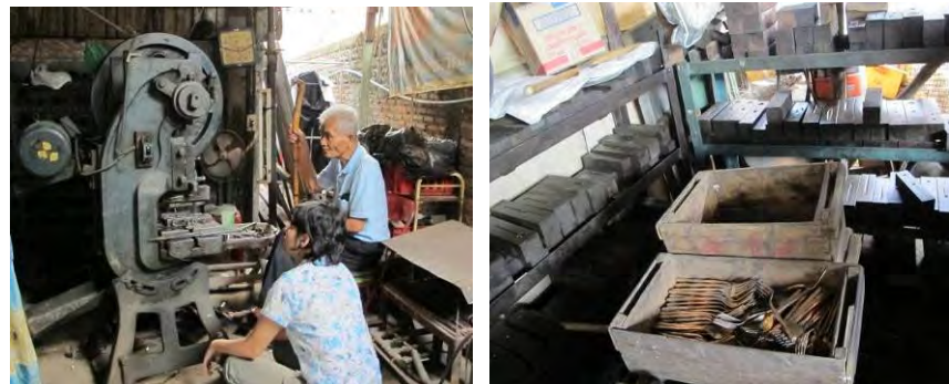
Figure 38: Pressing machine and the pressing mold
