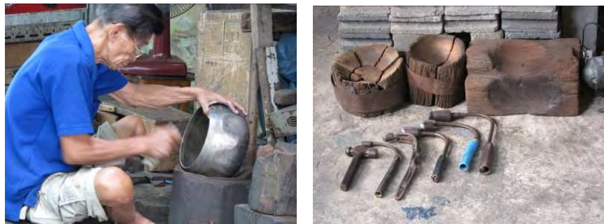
Figure 54: The hammering technique and its special tools.
