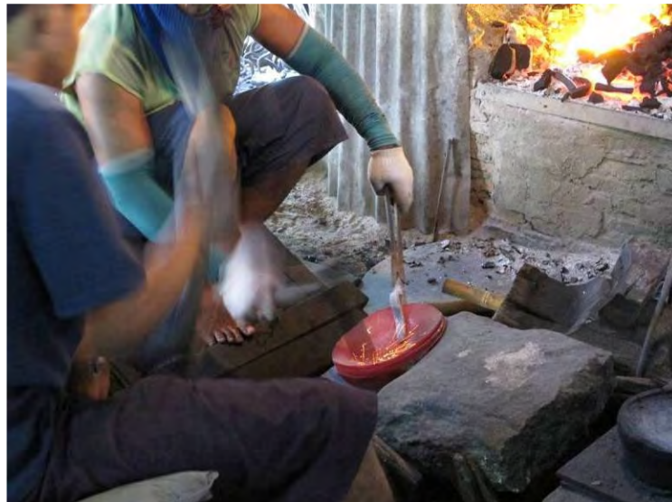
Figure 26: Two craftsmen are beating the metals as they were heated to a proper temperature.
