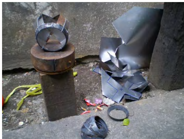
Figure 49: The rim of the alms bowl is attached to the cross steel.
