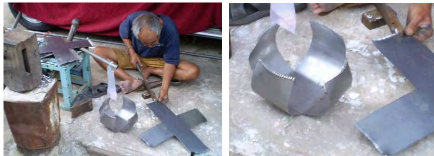
Figure 48: The cross steel making.
