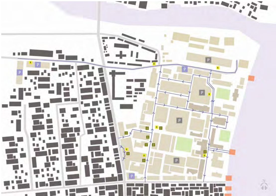
Figure 87: Car traffic direction, parking areas, proposed patient drop-off zone, and proposed shuttle bus stop area at Siriraj Hospital. Cars should be removed from in front of the buildings by providing parking areas and schedule shuttle bus services to reduce traffic congestion in the hospital.
