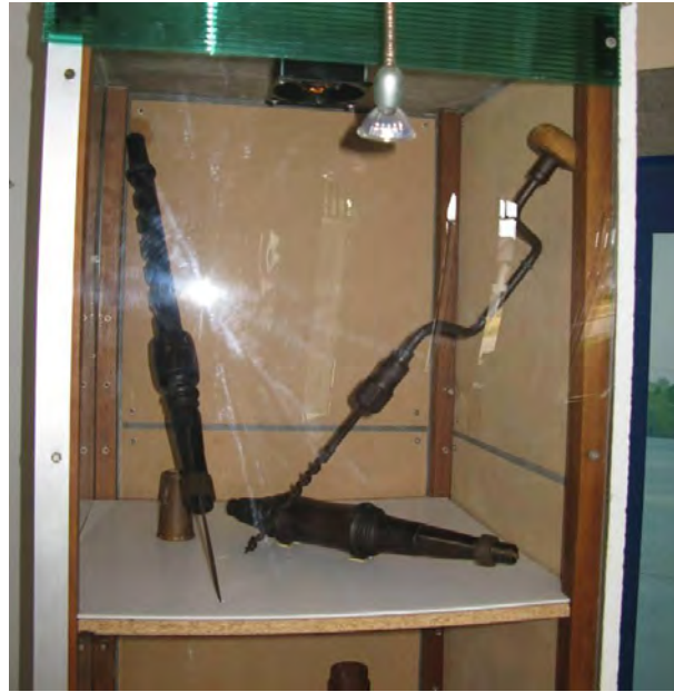
Figure 164 Woodworking tools. On the left is a hand drill in Chinese technology and on the right a hand drill in Dutch design which is today available for carpenters in central Thailand. These tools were available in Chantaburi ship dock, active in the late Ayutthaya to early Rattanakosin period. Photograph by Phungwong, N. on August 22, 2010.
