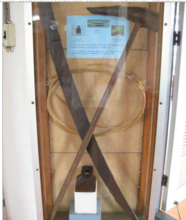
Figure 165 Woodworking tools saw and axe used to shape rough wood. These tools remain in boat making technology until today. This dock was active in the late Ayutthaya to early Rattanakosin period. Photograph by Phungwong, N. on August 22, 2010.
