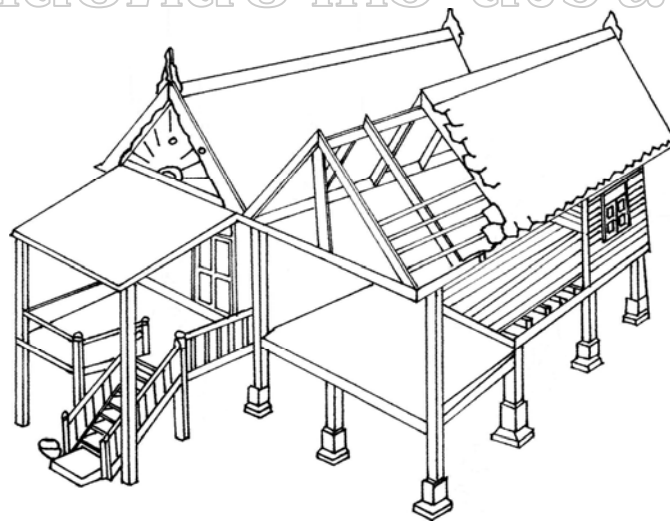
Fig.28 Structure of Southern house
