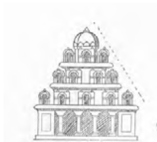
Fig.32: Indian Buddhist Viharn; Note the various stages with cells around them, a characteristic to be traced in the superstructure of many buildings of the farther India countries.
