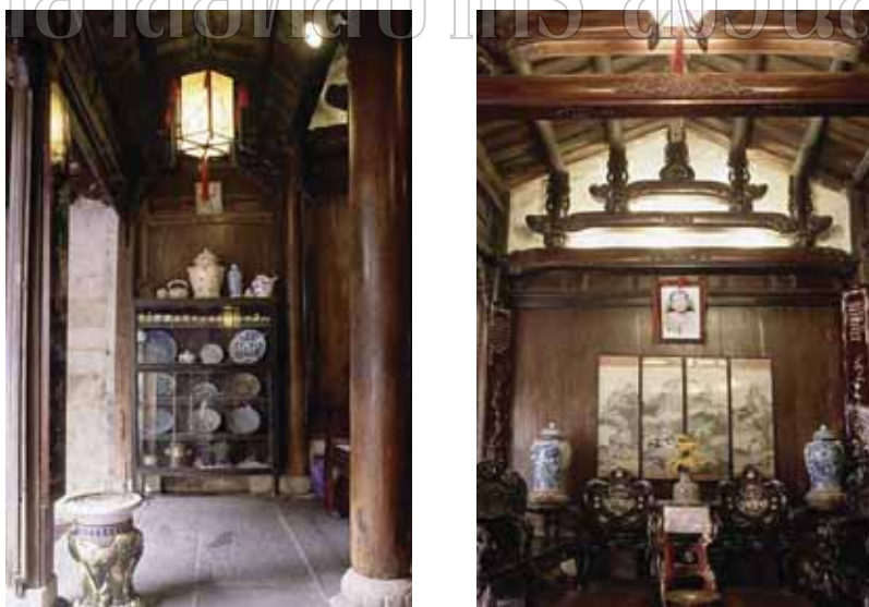
Fig. 45 A narrow intermediary space between the room at right and the courtyard at left. The arched wooden roof is an unusual feature rarely seen in traditional Asian architecture.
